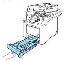
While pressing the green paper-guide release lever (1), slide the paper guides to fit the paper size. Make sure that the guides are firmly in the slots.
